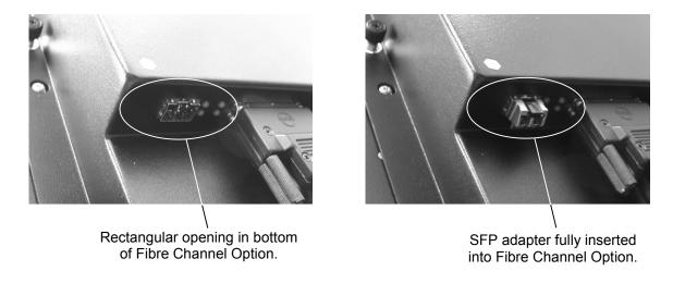
Figure 6-17 Inserting SFP Adapter into Fibre Channel Option
